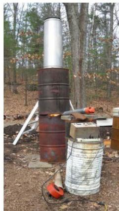
Fig. 12 - Artisanal biochar and heat production system made by Jolly Roger
