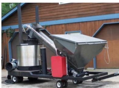
Fig. 13 - Heat and biochar production installation type HYBRID 250
