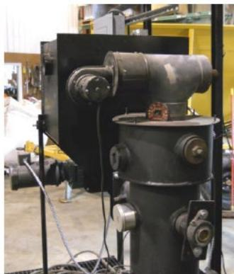
**Fig. 6 - The burner for hot air production of DRAGON type installation**
